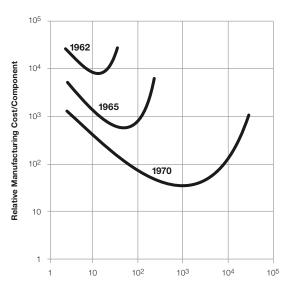
Number of Components Per Integrated Circuit
